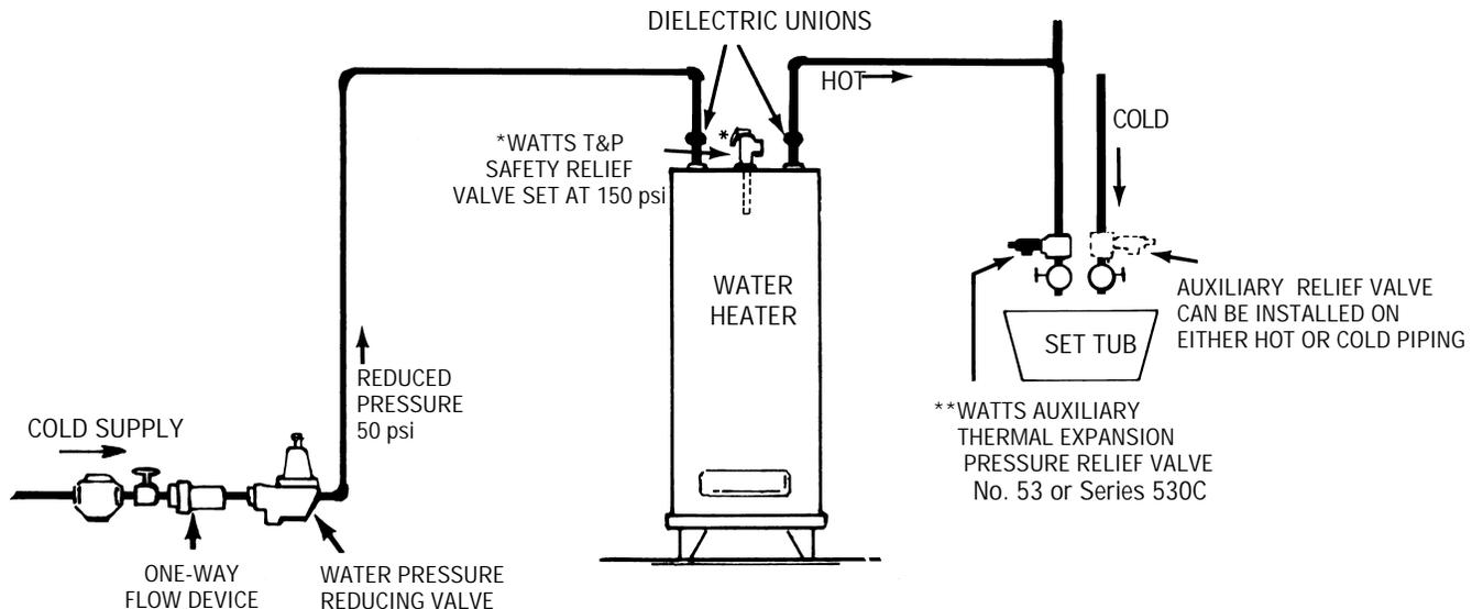
\*T&P valve should be set according to tank working pressure or local code requirements.
